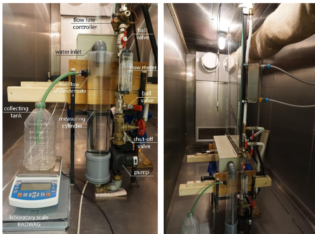
Fig. 2 Measurement system of water wall
