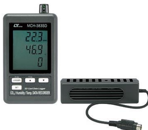
Fig. 4: Measuring device Lutron MCH-383SD
