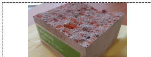
Fig. 4 Concrete sample with building debris
